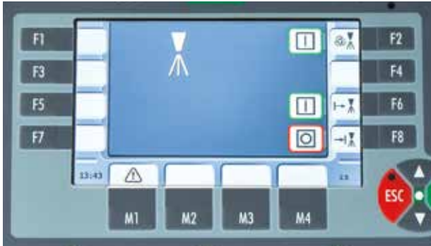
"Start of Job" and "End of Job" The convenience functions "Start of Job" (F6) and "End of Job" (F8) are provided so that spraying always starts and ends at exactly the required point and continues over full pave width.
